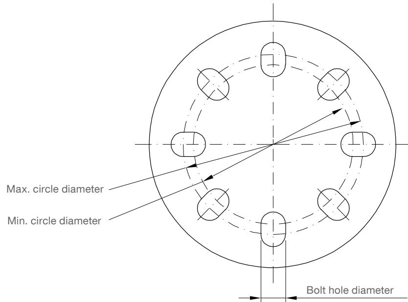
Universal flange (plane flange and Easy aimer flange) mates with bolt hole pattern of:
